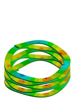
The image above shows the normal stress distribution in a wave spring from an FE analysis. As shown, a wave spring also uses the end coil, which makes it possible to reduce the building lengths.
